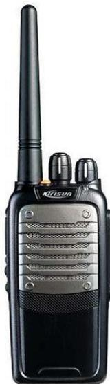
The Kirisun PT568 is a solid, robust and reliable radio offering the highest power and best outdoor range of any of our hire radios. It has 5 watts power output – the highest generally available on a walkie-talkie. It has a strong spring-loaded belt-clip on the back.
