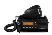
These radios can be used either mounted in vehicles or else set up as a "base station" for a group of mobile radio or walkie-talkies users.
