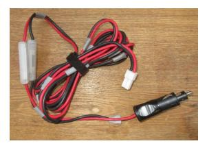
The vehicle radios do not need any kind of "installation" in the vehicle – the power lead just plugs in to the 12 volt "cigarette lighter" socket found on most cars, vans etc, and the magnetic aerial will attach to the roof of any steel-bodied vehicle.
